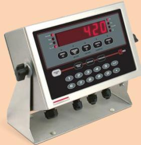
The 420 Plus is a single-channel digital weight indicator housed in a NEMA Type 4X/IP66-rated stainless steel enclosure. The indicator front panel consists of a large (.8 in, 20 mm), six-digit, and seven-segment LED display and twenty-one-button keypad. Features include:
