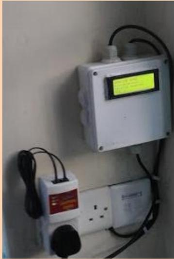
Bytronics Web Weight Indicator module is a hardware interface module that allows any web application to receive weight data from any digital weight indicator with rs232 communication support. The module has a configuration for setting up a web page that receives the weight data.
